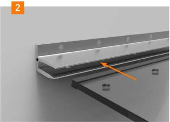
Align the glass panel and secure it with glass fixings.
