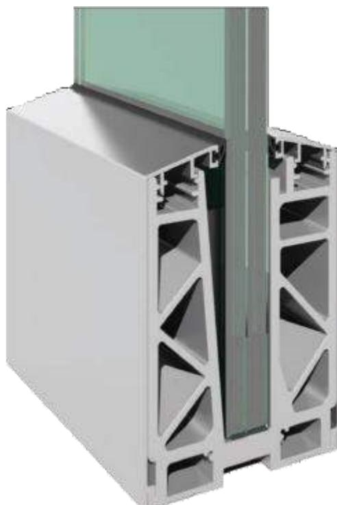
Baufit Elegant BS50 type glass railing is designed for 21,52 mm glass applications and it's glass supporting depth is 100 mm. Baufit Elegant BS50 features in your prestigious projects with it's safety increased design,easy application and aesthetic view.
