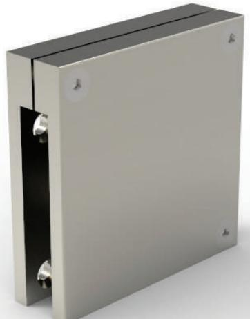
Vista series means aesthetic and minimalist details. Vista 100 is the best solution for narrow balconies which is serving newest, minimalist, aesthetic, simple and economic glass railings to your projects. Just fix the V100 glass holders to the four points of wall, put the glass inside the holders and close the holders with screws on it. The holders are suitable for 4+4 mm and 5+5 mm glass thickness.
