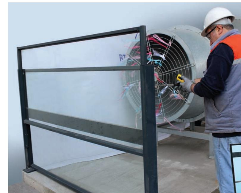
**Wind Tunnel (Wind Load)**
