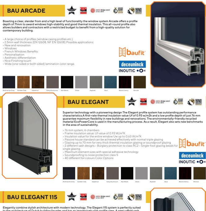
to the architecture of Dutch building façades and has an impressively slim profile view. A semi-offset sash emphasises the classical appearance and the choice of 50 colours also opens up a wide range of configuration options.The frame has an overall mounting depth of 115 mm and an incline of 5° or 15°. The inclined sash further enhances the retro look. Our extensive palette of 50 decors and colours offers a wide range of configuration options.
